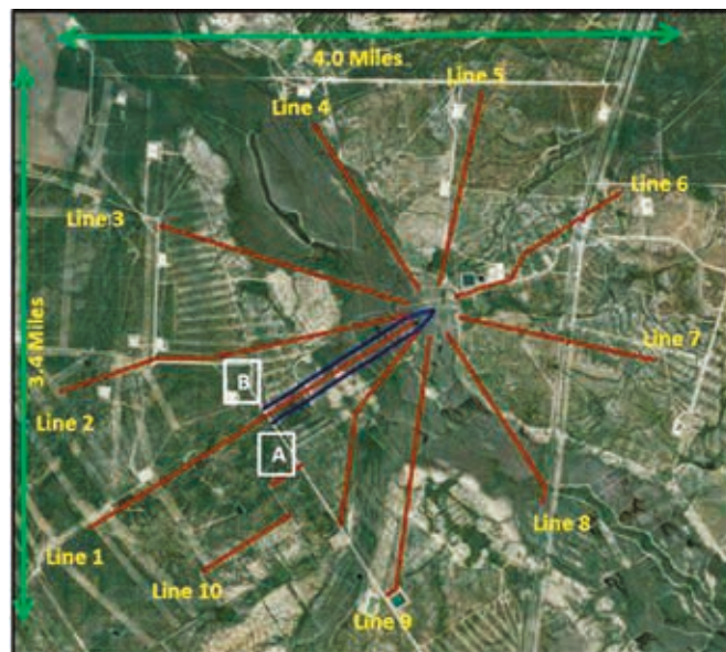
Figure 4. Map view of microseismic surface array. Radial lines of altogether 7200 geophones can be seen in red. Wellbores A and B can be seen in blue.
