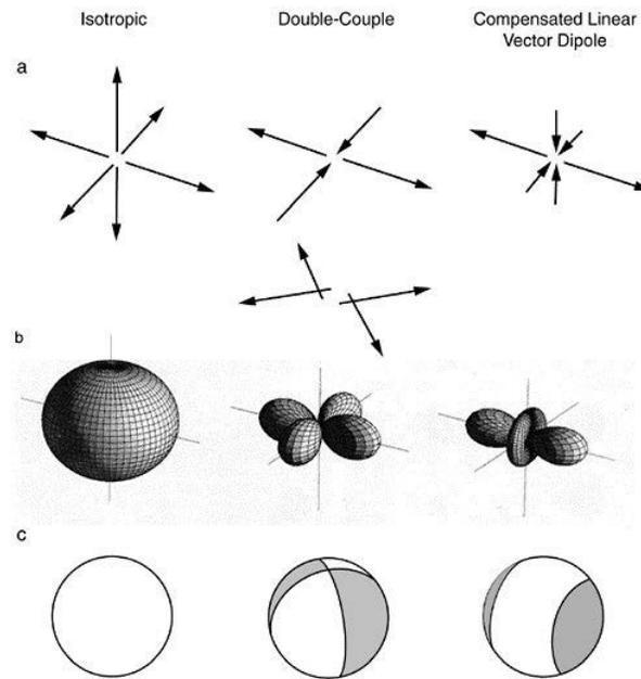
**Figure 10.** Source mechanisms for isotropic, double-couple and CLVD deformation. (Modified from Julian, Miller and Foulger, 1998)
