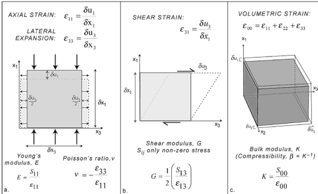
**Figure 2.** Schematic illustration of the relationships between stress, strain and the physical meaning of elastic moduli in different types of idealized deformation measurements. *Source: Zoback, 2010*
