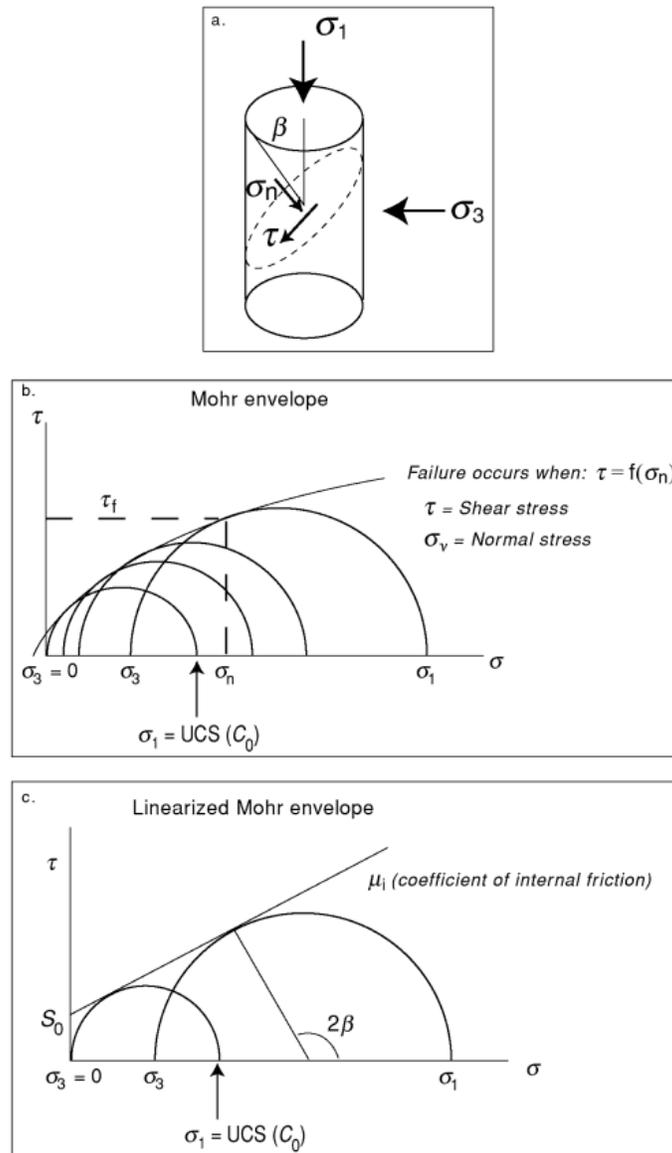
**Figure 5.** a) Diagram of a sample after a triaxial strength test. b) The Mohr envelope determined from several tests performed at different confining pressures. c) The linearized Mohr envelope.
