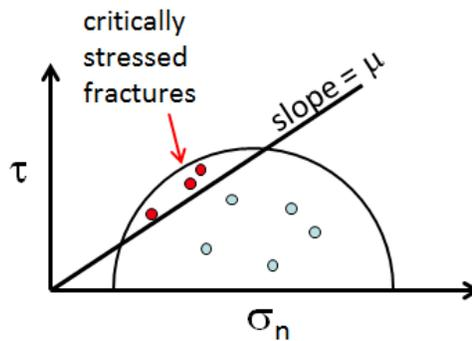
**Figure 9.** Mohr diagram showing the failure envelope for slip on pre-existing natural fractures.
