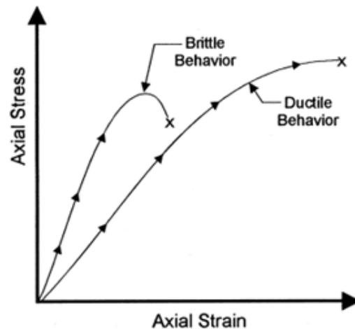
Figure 4. Schematic of brittle versus ductile rock behavior.
