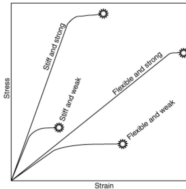
**Figure 13.** Idealized stress-strain behavior of materials with varying relative properties. *Source:* <http://www.geol.umd.edu/~jmerck/geol100/lectures/21.html>
