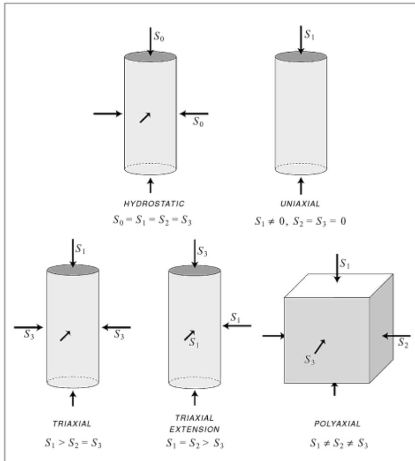
**Figure 3.** The most common types of rock mechanics tests and relative values of the stresses applied. Source: Zoback, 2010
