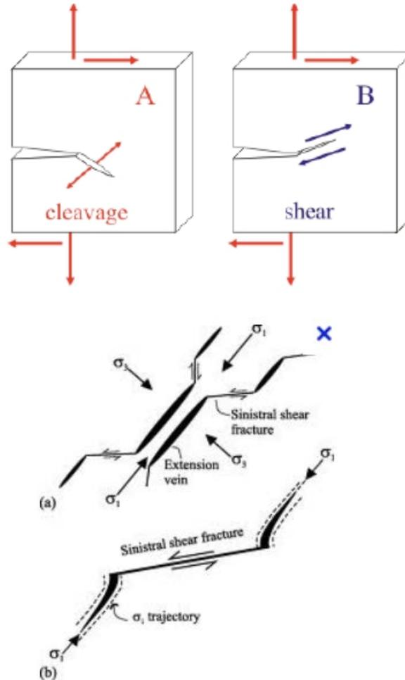
**Figure 14.** Potential mechanisms for mixed mode fracture propagation. (top - [http://www.kokch.kts.ru/me/t2/SIA\\_2\\_Fracture\\_Mechanics.pdf](http://www.kokch.kts.ru/me/t2/SIA_2_Fracture_Mechanics.pdf); bottom - <http://emg.geoscienceworld.org/content/13/1-4/129/F9.expansion.html>)
