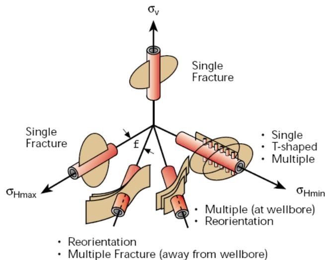
**Figure 12.** Illustration of various possible (simplified) hydraulic fracture geometries and their dependence on the orientation of the borehole with respect to the principal stresses. *Source: Barree & Associates*
