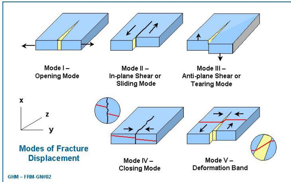
Figure 6. Fracture displacement modes. Source: [www.makel.org](http://www.makel.org)
