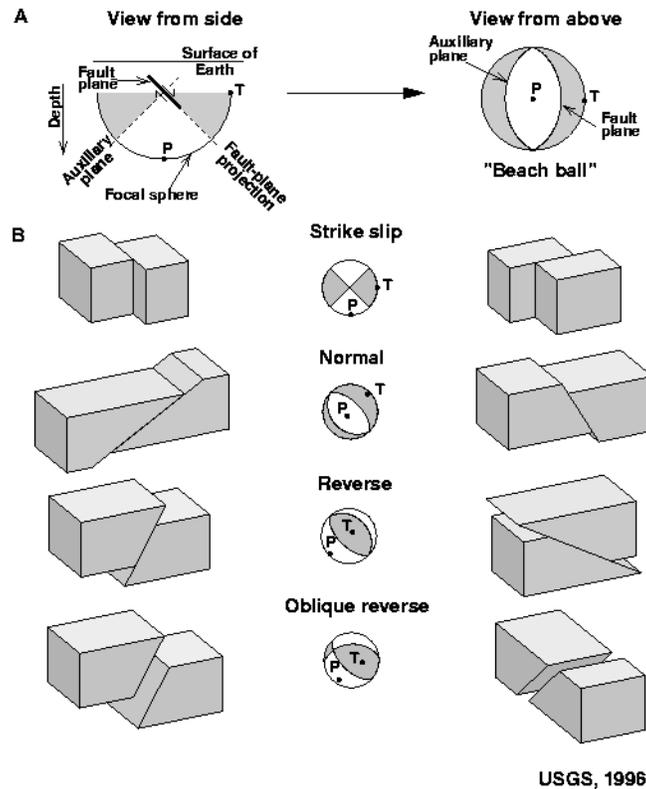
**Figure 11.** Schematic diagram of a focal mechanism for different fault types.
