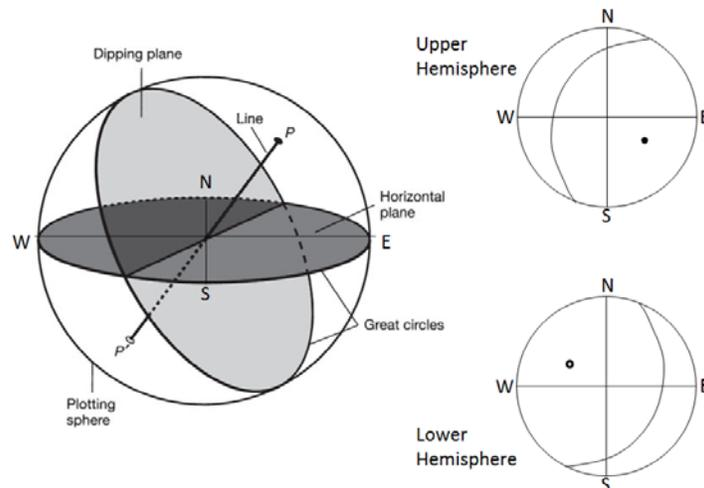
**Figure 8.** How planar features and their poles are represented on 2-D stereonet plots.
