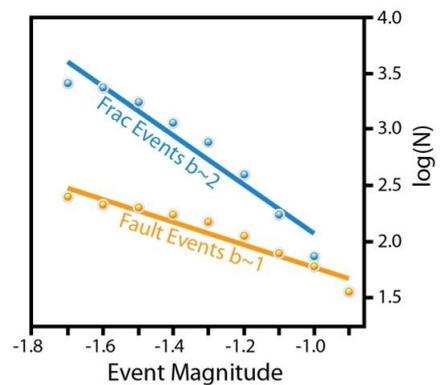
**Figure 2** Blue line with a slope of 2.2 represents the fracture induced events with 40/90/-125 strike, dip and rake ( $s$ - $d$ - $r$ ) respectively. Orange line with a slope of 1.0 is the fault reactivation events with 240/80/10  $s$ - $d$ - $r$ . Magnitude values are shown in the axis and number of events are shown in the y axis in hundreds.
