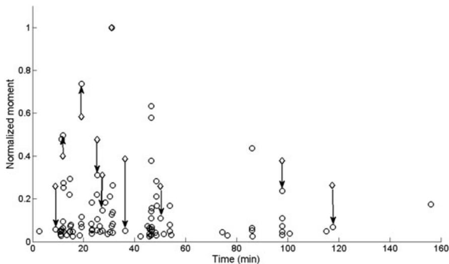
**Figure 5** Relative seismic moment versus origin time for surface (black circles) and top ten downhole (black diamonds) events. The seismic moments of the largest event from surface and the largest event from downhole were scaled to 1 and their relative origin times adjusted to match. Corresponding matches of the remaining 9 events are represented by the black arrows. Horizontal axis shows time in minutes since beginning of the fracturing.
