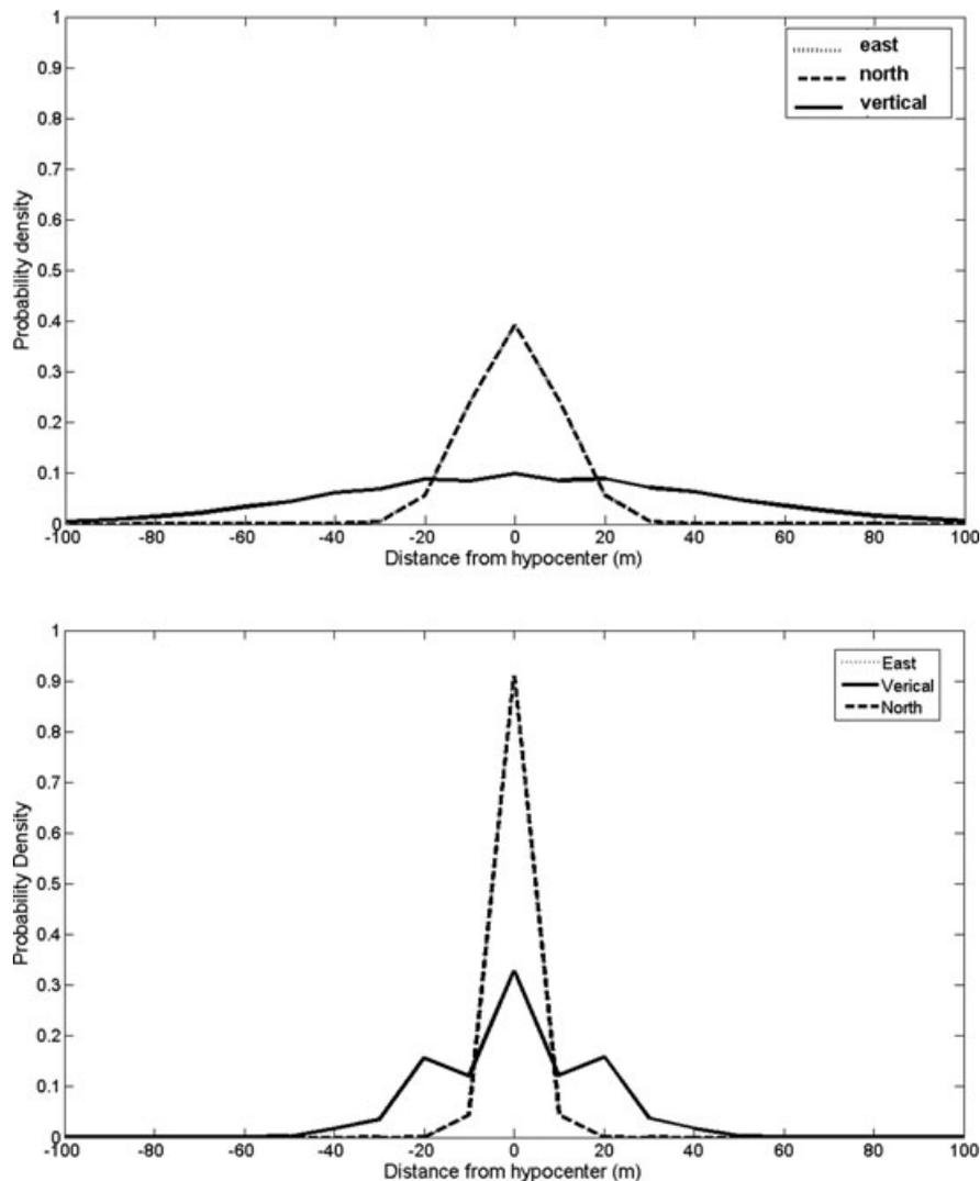
**Figure 2** Marginal probability density functions of a hypocenter located 3000 m below the centre. We used standard deviation of 10 (top plot) and 4 ms (bottom plot) for arrival times of P-waves. An array of 121 receivers at the surface with offset to depth ratio approximately 1:1. The solid and dotted lines overlay as these probabilities are exactly the same.
