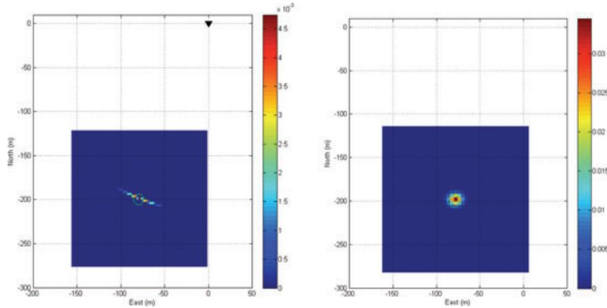
**Figure 7** Map views of a probability density function for a hypothetical microseismic event located at  $-80$  m east and  $-200$  m north coordinates from a vertical borehole array at  $0,0$  (left plot) and surface array (right plot). The vertical borehole array is represented by black triangles in the north-east corner of the left plot.
