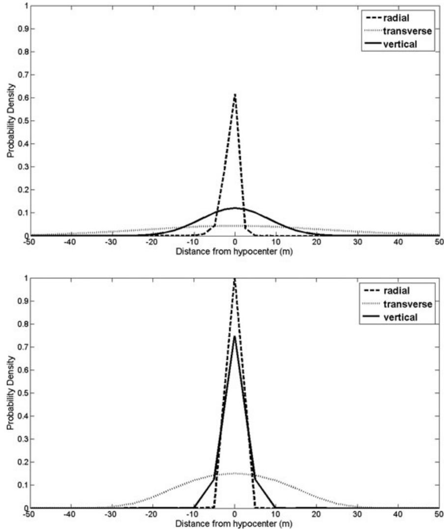
**Figure 1** Marginal probability density functions of a hypocenter located at the central depth of a monitoring array at a distance of 300 m. Both panels represent vertical monitoring arrays at 300 m horizontal distance from hypocenter, top panel represents 5 receivers spanning 120 m, bottom panel represents 11 receivers spanning 300 m. We used a standard deviation of 1 ms for arrival times and  $10^\circ$  for the backazimuth.
